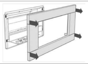
Reverse these steps to re-fit the Fascia, ensuring the two connections are correctly plugged in by testing the fire.
