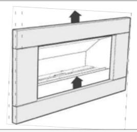
Now slide the fascia towards you until it falls into the additional slot, unplug the electrical cord. Nowyou can rest the Fascia on the ground.
